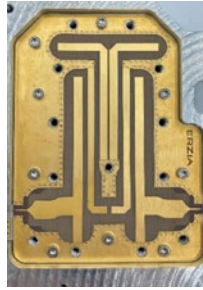
Figure 11: ERZ-BPF-0190-0210-1.8 bandpass SSS filter
